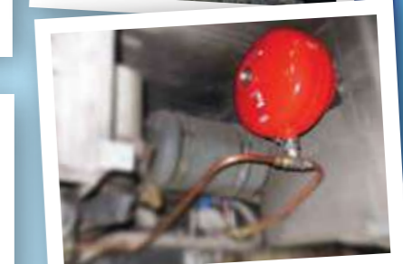
Typical IPEX installations in bus engine compartments, Australia.
